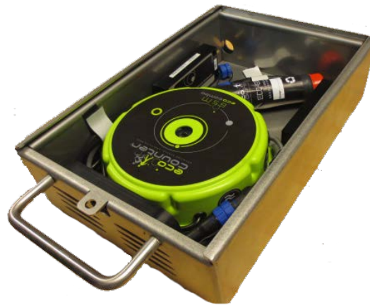
Figure 11. Stainless Steel Box that Houses the Tube Counter.
